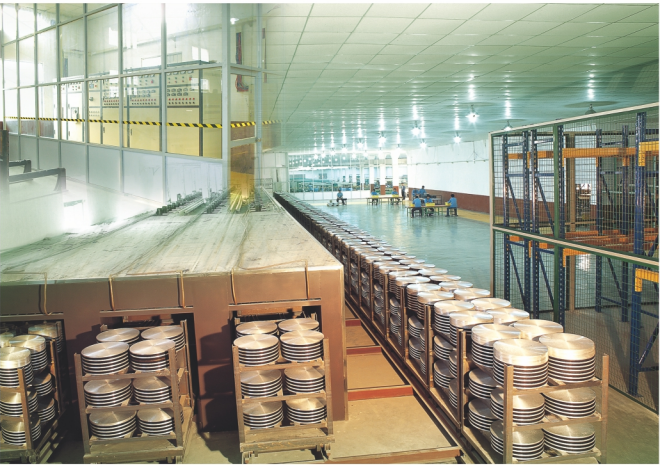
24小时自动控制隧道窑 24 hours computer system controlled the tunnel kiln
